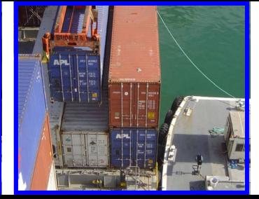
Crane Operators: be especially careful when handling containers in stacks next to a bunker barge
