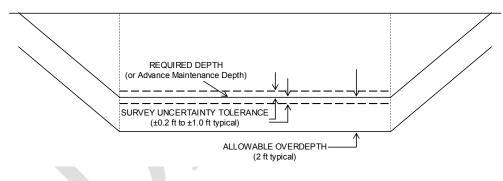
Figure 2. Survey uncertainty tolerances in soft bottom maintenance dredging projects
