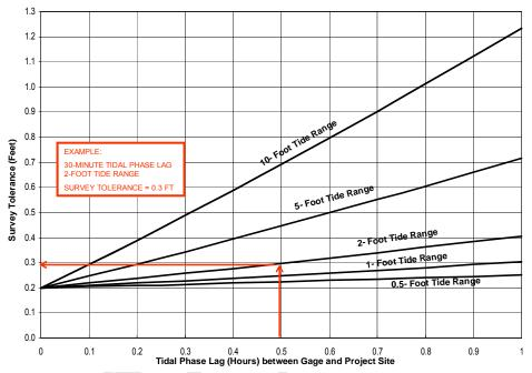
more can occur over relatively short distances (less than one-half mile) during ebb or flood tides when gage readings are extrapolated to the project area. Carrier phase RTK methods are the only effective way to minimize or eliminate these tidal phase errors, and minimize the resultant Survey Tolerance value.
