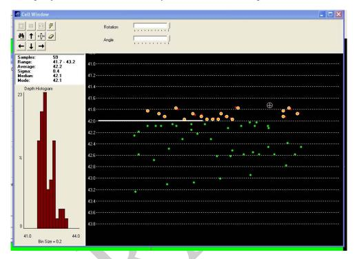
may be estimated based on the standard deviation of the mean. Estimates of the uncertainty of the mean or average depth in the cell relates to the "survey tolerance" used in evaluating clearance.
