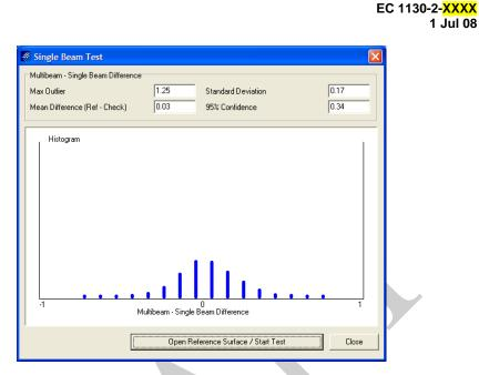
Figure A-4. Comparison of a multibeam system (S/V Shuman) against single-beam reference surface from a different vessel (S/V Cherneski)—Philadelphia District. The multibeam was 0.03 ft deeper with a 95% standard deviation of ±0.34 ft as compared to the assumed absolute single-beam reference
