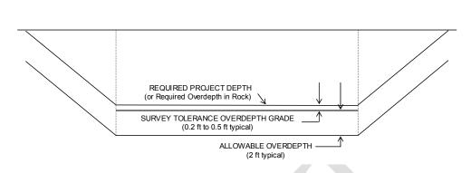
Figure 1. Survey tolerance overdepth grade in hard bottom projects (rock, dense clay, or manmade materials)
