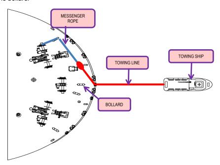
[Step 4] Connect the rope stopper between the towing line and the bollard.
