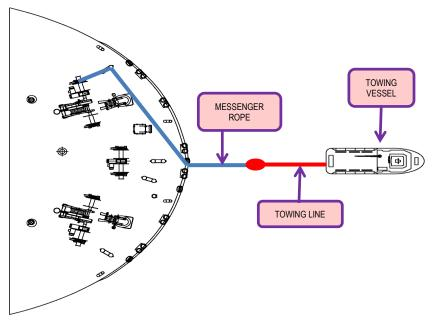
**[Step 3]** Wind the messenger rope by using warping head until the eye splice of the towing line reaches the bollard.
