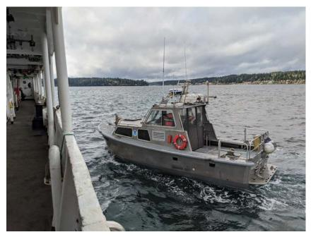
Survey launch that will be doing the majority of survey work, especially in shallow waters and nearshore, etc.
